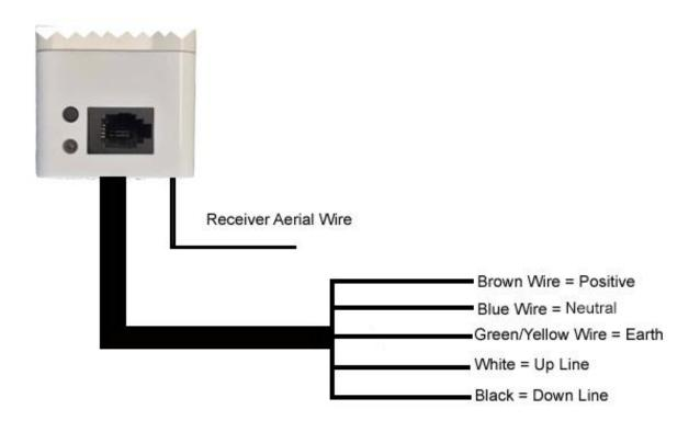
The DT980TV/S Hard Wire Curtain Track motor is wired directly into the power supply using the Brown, Blue and Green/Yellow wires (please see above for wiring details).
